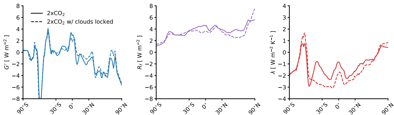
Supplemental Figure 5: GCM feedback locking. Zonal-mean profiles of ocean heat uptake ( G' ), radiative forcing ( R_f ), and the net radiative feedback ( \lambda ) from the CESM1(CAM5) abrupt2xCO 2 experiments with (solid) and without (dashed) cloud radiative effects.
